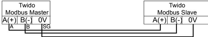
The wiring in this example demonstrates a simple point to point connection. The three signals A(+), B(-), and 0V are wired according to the diagram.
